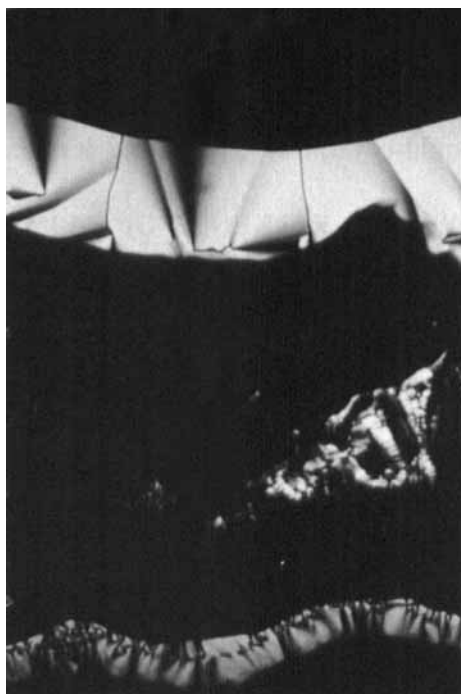
Figure 1. Contact preparation between glucamine and 4- n -octadecyloxybenzoic acid. Area is approximately 0.6 \times 1.0 \text{ mm}^2 , T = 140.0^\circ\text{C} , crossed nicols, with cover slide, \lambda/2 -plate. Bottom, isotropic phase, acid 321 ; between, columnar discotic phase, salt + acid; middle, S_A phase, salt 122 ; between, columnar discotic phase, salt + amine; top, isotropic phase, amine.
